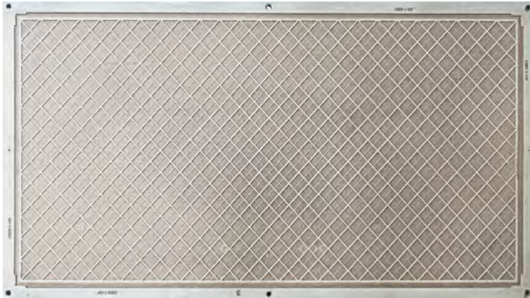
Figure 2.31. Laser engraved back side bakelite pattern
