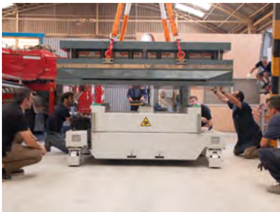
Figure 6.15. Transport of the mould for installation or replacement.
