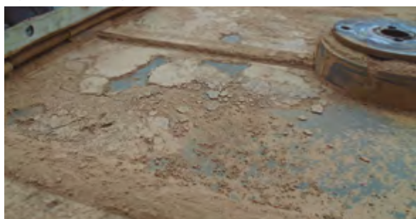
Figure 7.7. Atomised powder between bench plate and ejecting plate due to bellows rupture.
