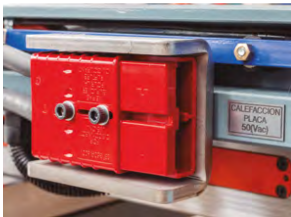
Figure 3.66. Fast plugs on an upper plate.
