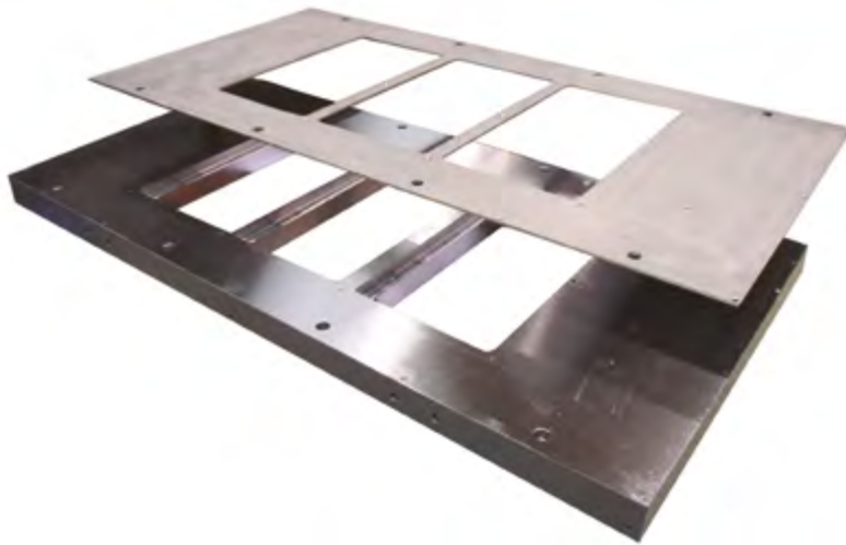
Figure 3.20. Wear resistant plate ready to be screwed onto the die box.
