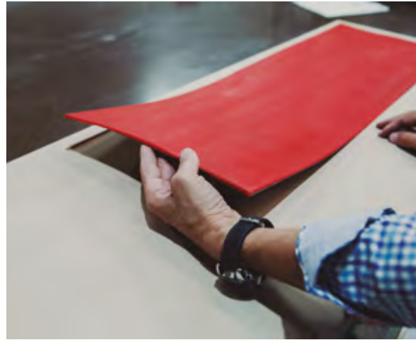
Figure 4.5 Rubber sheeting for punches.
