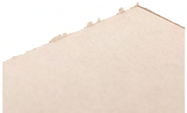
Figure 7.11. Burrs on the good face.
