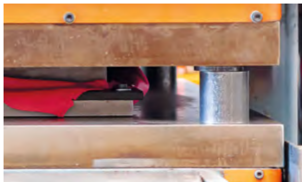
Figure 4.48. Arrangement of the stops in the press (detail).
