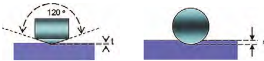
Figure III.4. Rockwell hardness test (diagram).
