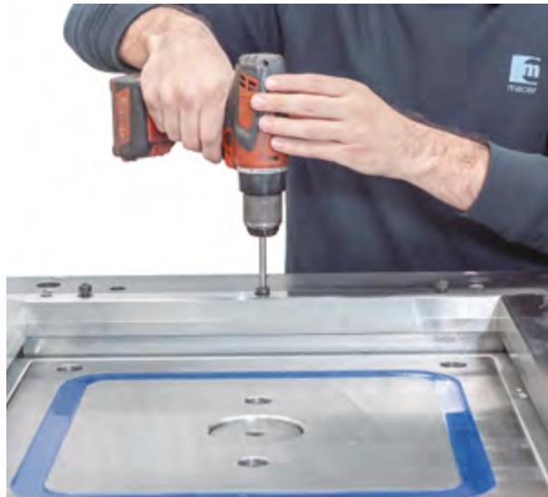
Figure 4.23. Set up process of the rectified interchangeable liners (3).
