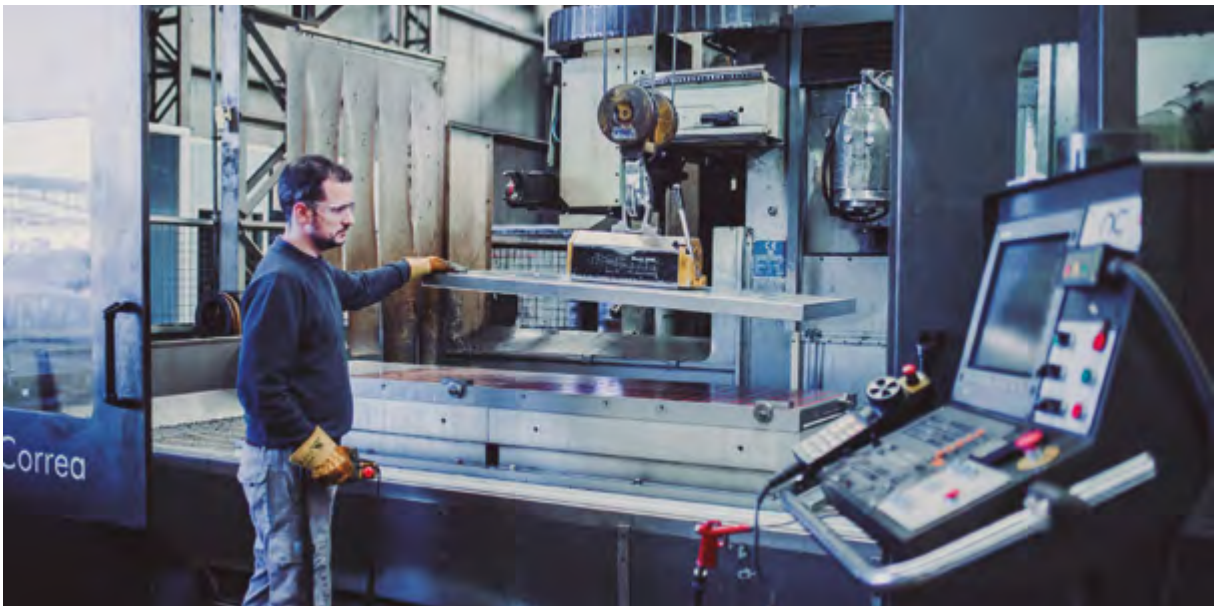
Figure 6.12. Lifting and handling of large loads with the aid of hoists and magnets.
