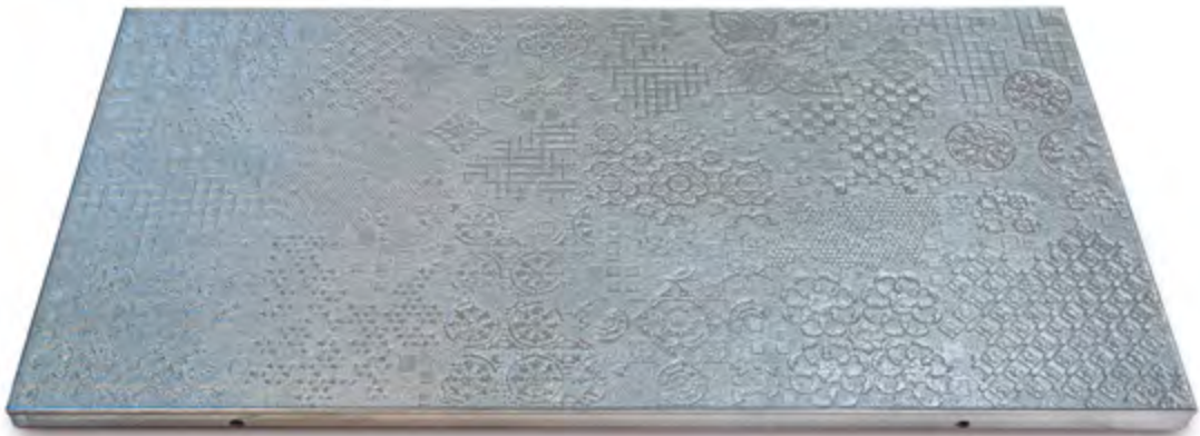
Figure 3.36. Punch for large format tiles (60 x 120 cm) with relief.
