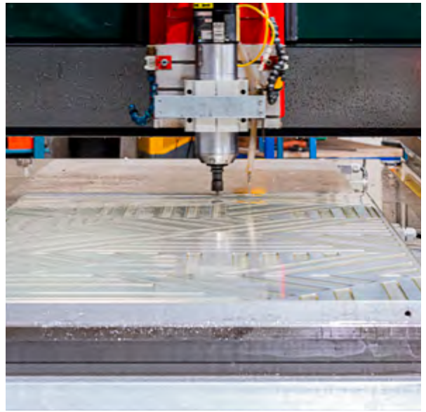
Figure 2.30. Relief machining with milling machine on aluminium pattern
