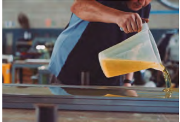
Figure 4.40. Liquid rubber pouring into a punch.
