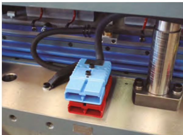
Figure 3.65. Fast plugs on the lower side of the mould.
