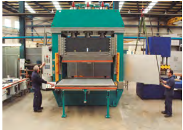
Figure 4.41. Six-piston press for applying the rubber coat to large-format punches.
