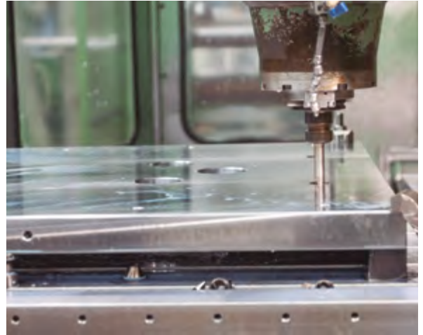
Figure 4.8. Rough milling of a bottom plate.
