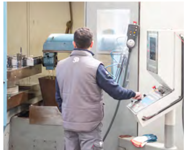
Figure 4.9. Drilling of the bench plate with a CNC drilling machine.
