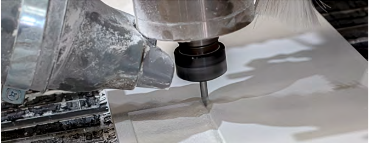
Figure 2.25. CNC milling machine for plaster prototypes.
