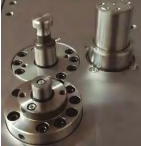
Figure 3.6. Detail of the SACMI SPE 2+2® forming and extraction system. Photo courtesy of SACMI.
