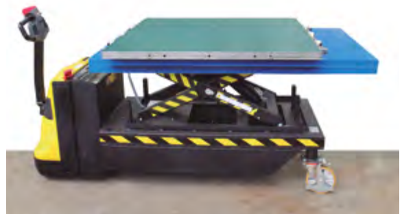
Figure 6.14. Manual hydraulic trolley for changing punches.
