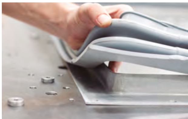
Figure 3.17. Elastomeric bellows with protective frame.
