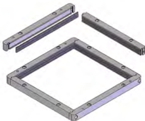
Figure 3.34. Drawing of tungsten carbide strip inserted into a liner and reinforced liners assembly
