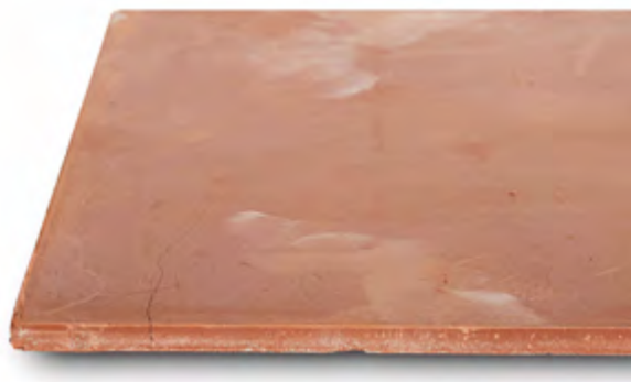
Figure 7.20. Crack caused by impact (in tiles with insufficient compaction).
