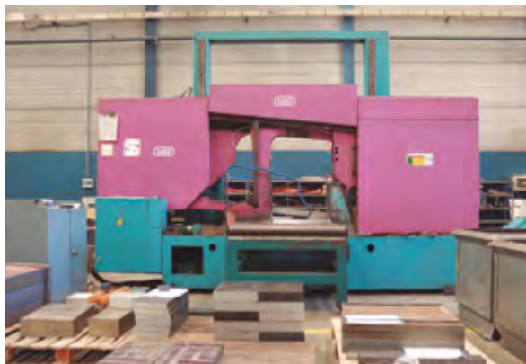
Figure 4.33. Cutting of the raw steel plates with a saw.
