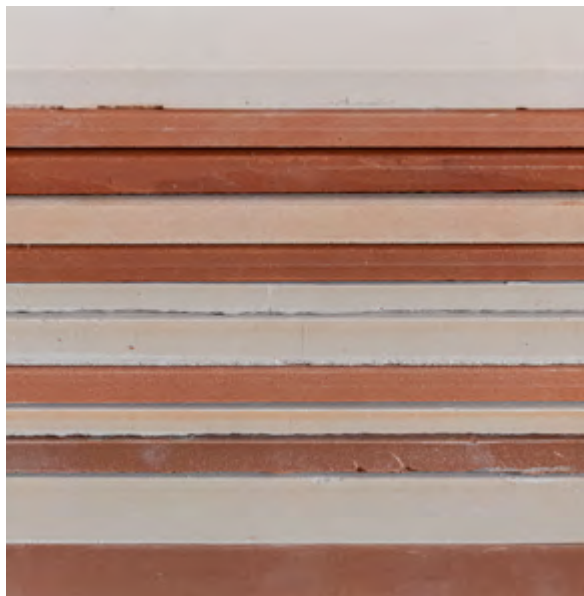
Figure 2.3. Tile sections with different thicknesses
