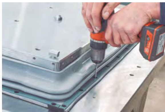
Figure 3.18. Silicone bellows assembly.
