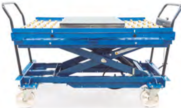
Figure 6.13. Manual hydraulic trolley for changing punches.
