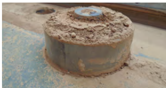
Figure 7.7. Atomised powder between bench plate and ejecting plate due to bellows rupture.
