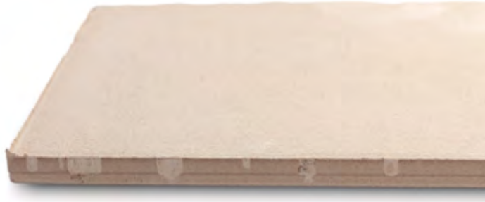
Figure 7.19. Side scratches caused by off-centre mould.
