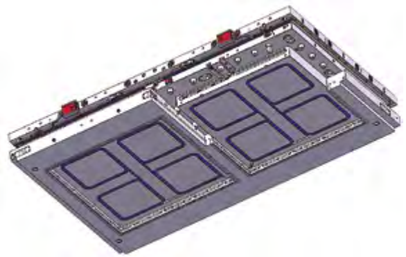
Figure 5.14. Mould equipped with hydraulically compensated upper plate.
