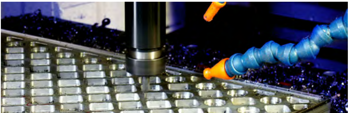
Figure 4.37. Machining of the oil compensation system in isostatic grid punches type MRPV.
