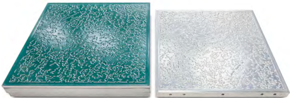
Figure 2.27. Back side relief on the aluminum pattern (right) and the corresponding punch (left)
